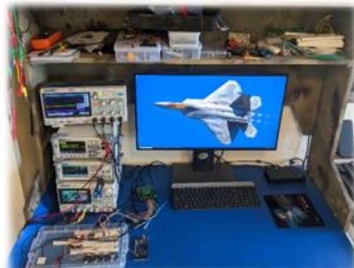
4Ch, 200MHz Oscilloscope, 30MHz Function Generator, 5.5 Digit Multimeter, 3GHz Nano VNA, Logic Analyzer, Linear Power Supply
